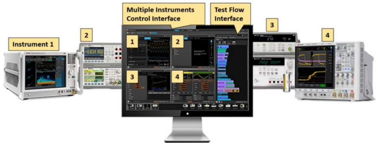
Figure 7. Multiple instruments integrated control with PathWave BenchVue complete control collection
