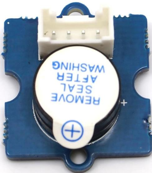
This is a simple yet enjoyable Grove to use. The piezo can be connected to digital outputs, and will emit a tone when the output is high.
