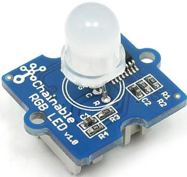
Chainable RGB LED is based on P9813 chip which is a full-color light source LED driver chip, and can provide constant current drive and modulated output of 256 gray.
