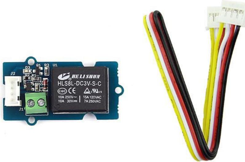
The Relay Grove is a digital normally open switch that controls a relay capable of switching much higher voltages and currents than your BBG boards. When set to HIGH, the LED will light up and the relay will close allowing current to flow. The peak voltage capability is 250V at 10 Amps.
