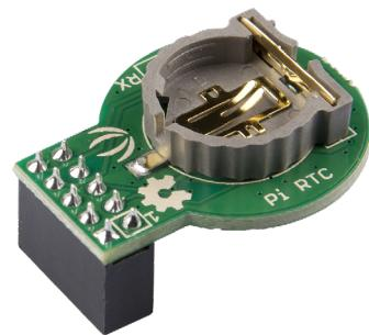
The Pi RTC tool detects automatic power-fail and incorporates switch circuitry. This module features programmable square-wave output signal and stores data through Non-Volatile (NV) RAM. The Pi RTC tool is available in 30mm x 23mm x 15mm dimensions and weighs about 13.2g.
