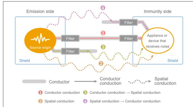
Aside from ensuring that the leads are adequately attached to the appropriate connection points and that the shielding is effectively connected, there are a limited number of methods to ensure that noise produced by the device won't be emitted from the leads and external noises will not be conducted into the device through the leads. EMI suppression filters are one of the most common and effective ways of attenuating noise and interference signals.
