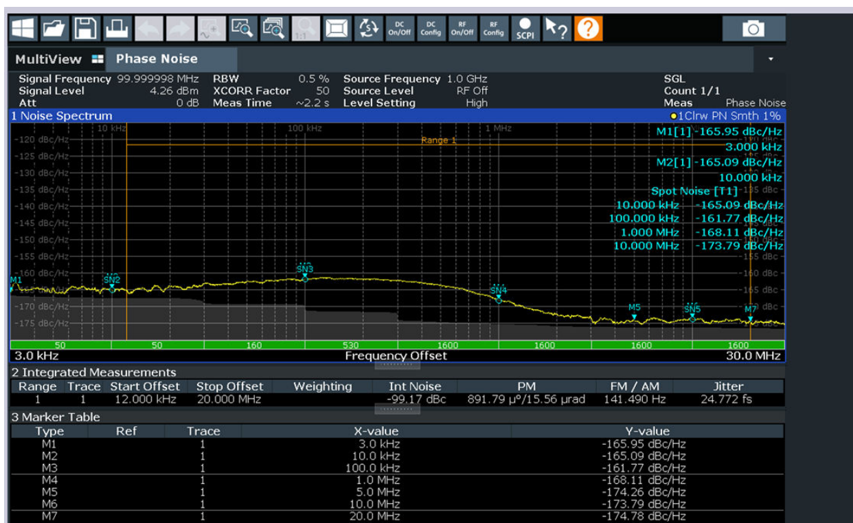
Figure 3-1. Clock Phase Noise of the 100 MHz Input Clock Generated with R&S SMA 100B
