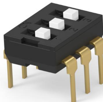
TE Connectivity's (TE) ALCOSWITCH Next Gen. DIP switch ADE and ADF series are designed for space-saving and streamlined manufacturing with high contact pressure allowing for aqueous cleaning without the need for tape sealing.
