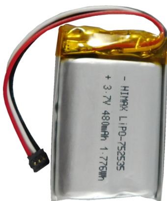
Figure 4. 480mAh 3.7V Li-Po Battery
