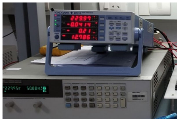
Figure 26. Standby power consumption: 0.21 W at nominal input voltage
