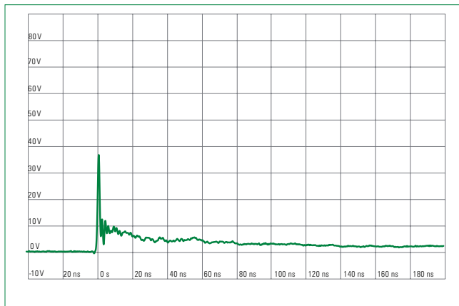
IEC 61000-4-2 +8 kV Contact ESD Clamping Voltage
