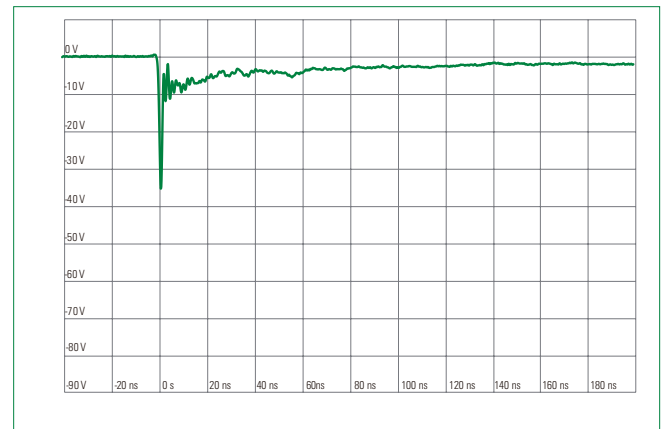
IEC 61000-4-2 -8 kV Contact ESD Clamping Voltage
