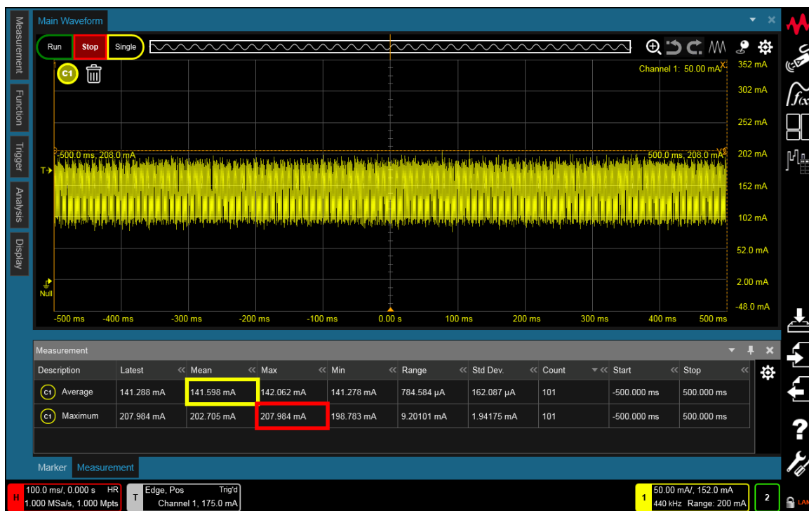
Figure 3. +5V Current consumption of iMXRT106L + Hyperflash + Microphones – Waiting for “hey NXP” wake word - large time window.
