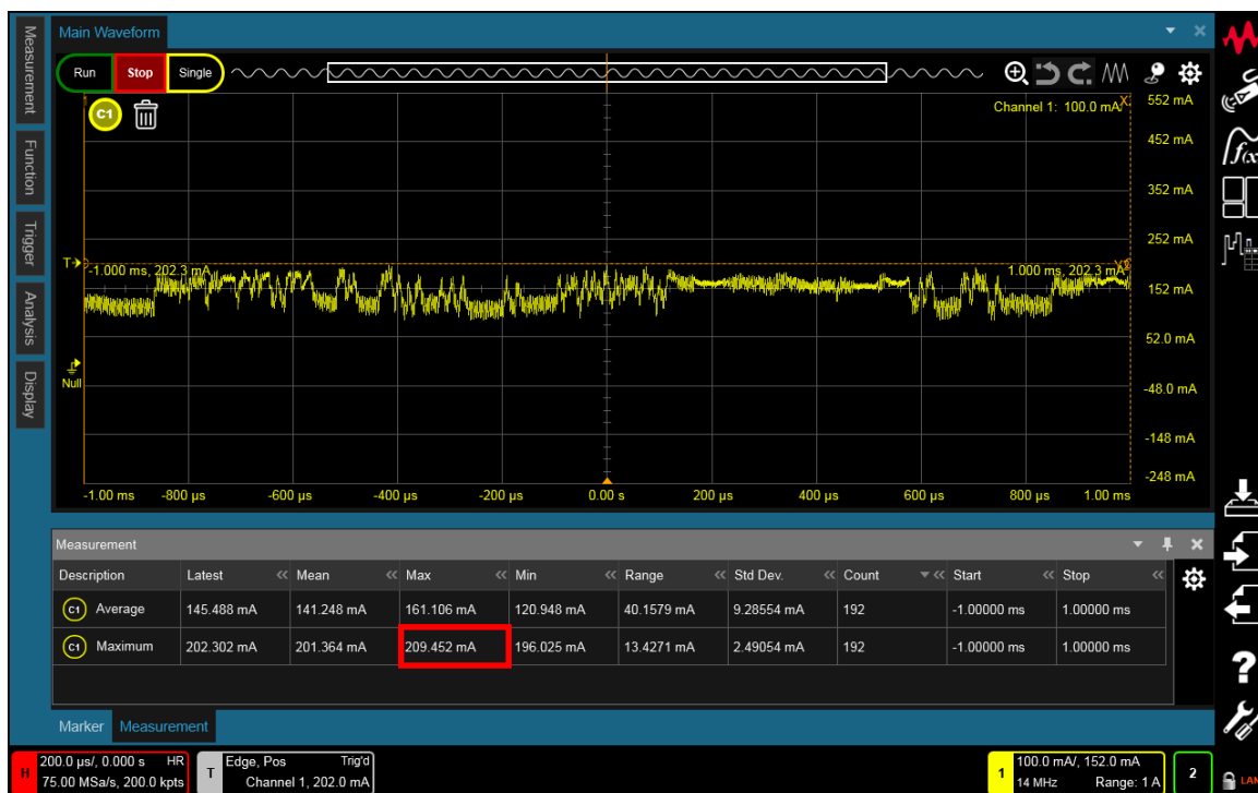
Figure 4. +5V Current consumption of iMXRT106L + Hyperflash + Microphones – Waiting for “hey NXP” wake word – zoom.
