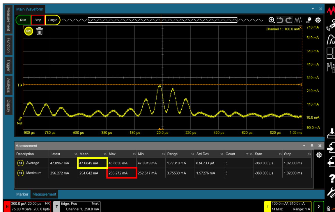
Figure 6. +5V Current consumption of Class-D audio amplifier – Saying “Sorry...”, with max volume, zoom on the current peak.
