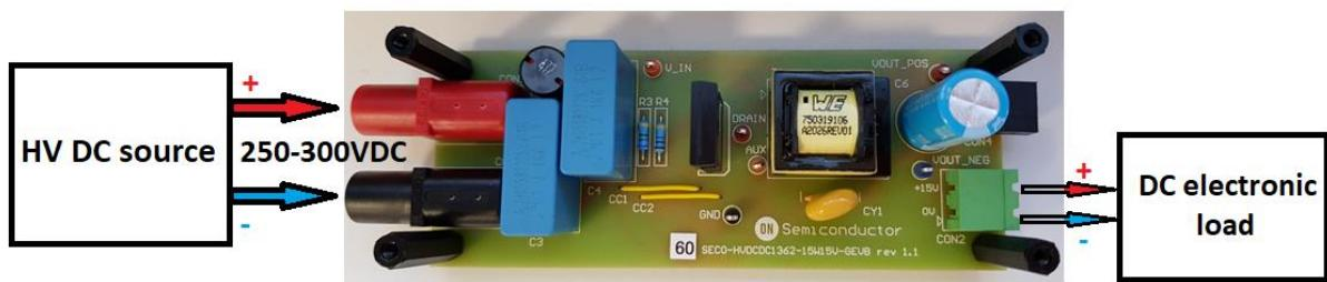
2. Turn on HV DC source and DC electronic load. Test is the following:
