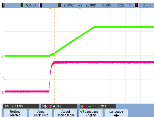
Figure 11. Vin Start-up Delay (CH2: Vout, CH1: Vin) (Vin=48V, Iload=0A, Cload=5500μF, Ta=+25°C, 20mS/div)
