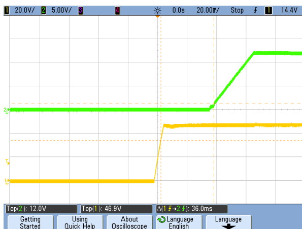
Figure 11. Vin Start-up Delay (CH2: Vout, CH1: Vin) (Vin=48V, Iload=0A, Cload=5500μF, Ta=+25°C, 20mS/div)
