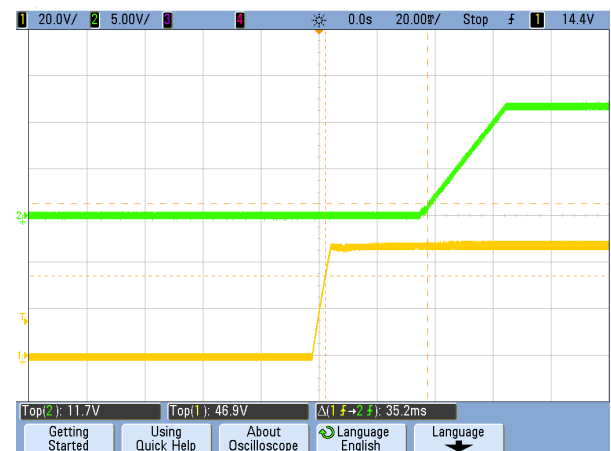
Figure 12. Vin Start-up Delay (CH2: Vout, CH1: Vin) (Vin=48V, Iload=33A, Cload=5500μF, Ta=+25°C, 20mS/div)
