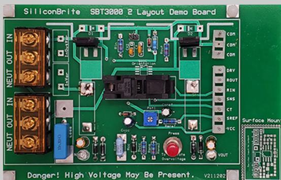
The SBT3000 Evaluation Module (EVB), is an engineering circuit board designed for testing the operation of the SBT3000 integrated circuit. The SBT3000 EVB contains an SO8 IC socket and all the necessary support components to be able to apply an input voltage and a moderate load in order to evaluate the overvoltage protection features of the device.
