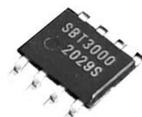
The robust solid-state solution features a unique architecture that automatically detects AC line over and under-voltage conditions and safely isolates the power line from the load until the AC input voltage is within its normal range. The SBT3000 can also be used in conjunction with a varistor to provide superior and unmatched line voltage protection.
