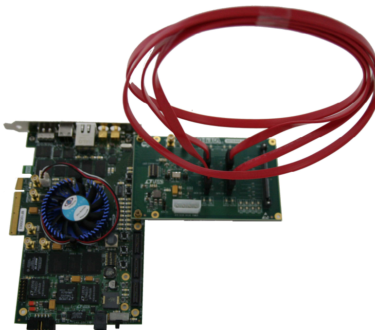
Figure 4.5 SATA loopback ribbon cable connection
