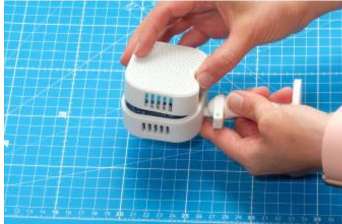
**Step 5.** Finally, position the cover over the board and press it down until all snaps engage securely.
