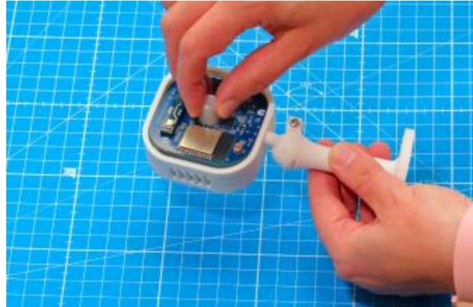
**Step 2.** Insert the IQ board into the chassis, ensuring it is properly seated on the spacers.
