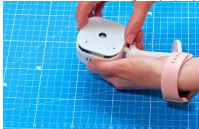
**Step 3.** Attach the front lid by pressing it until all the snaps click securely into place, ensuring that the holes on the front lid are positioned on the left as shown in the picture.
