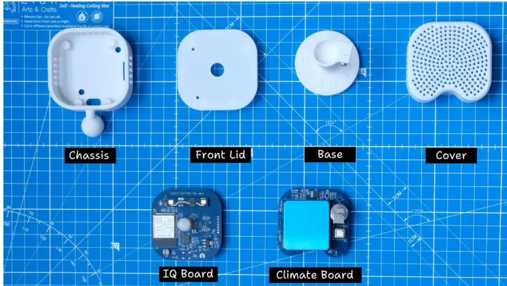
A key feature of the enclosure design is its simplicity, with all components fitting together seamlessly to ensure straightforward and efficient assembly.
