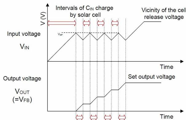
As soon as there is sufficient energy available on the input side, the buck DC/DC Converter will be enabled to transfer energy from input to output until the energy drops below a threshold. This process repeats and increases the voltage in the energy storage device until the required level is reached.
