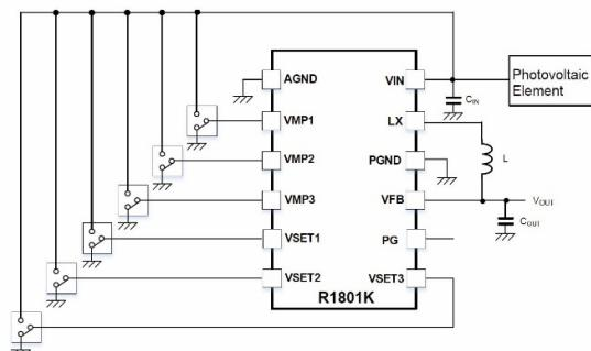
initial voltage setting increases or decreases in a 100mV step, the total adjustable range is  $\pm 300\text{mV}$ .
