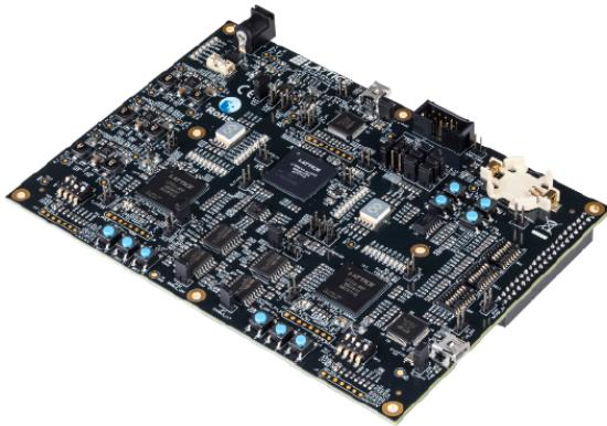
MachXO3D adds an immutable embedded security block, enhanced control functions, expanded user flash memory up to 2700 kbytes, and available in Commercial, Industrial and AEC-Q100 qualified Automotive grade.
