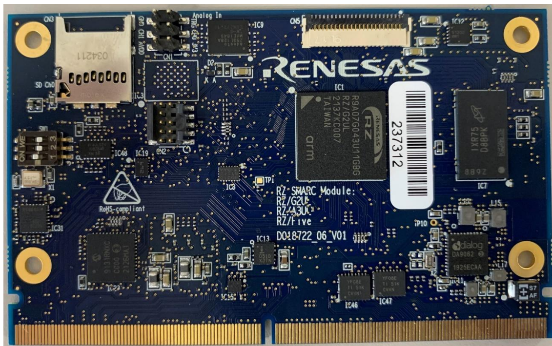
Figure 1.2 Top View of the RTK9743U11C01000BE
