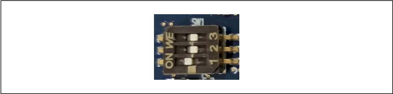
Figure 3.9 Default Setting of System Setting DIP Switch (SW1)
