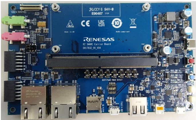
Figure 5.2 Top View of the RZ SMARC Series Carrier Board
