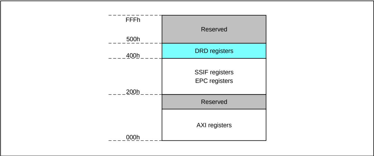
Figure 35.4-2 AXI Address Space for DRD Registers in DRD Mode
