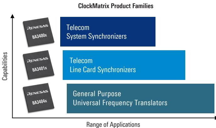
In the ClockMatrix family, the Universal Frequency Translator (UFT™) devices perform jitter attenuation and frequency translation functions for general purpose applications.
