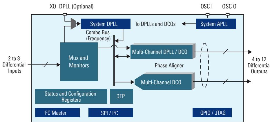
ClockMatrix devices include two types of timing channels: Digital PLL / Digitally Controlled Oscillator (DPLL/DCO) channels and DCO only channels. Any DCO can free run based on the local oscillator. They can be controlled by external software or they can be connected to a DPLL channel to supply additional outputs and frequencies for that DPLL.
