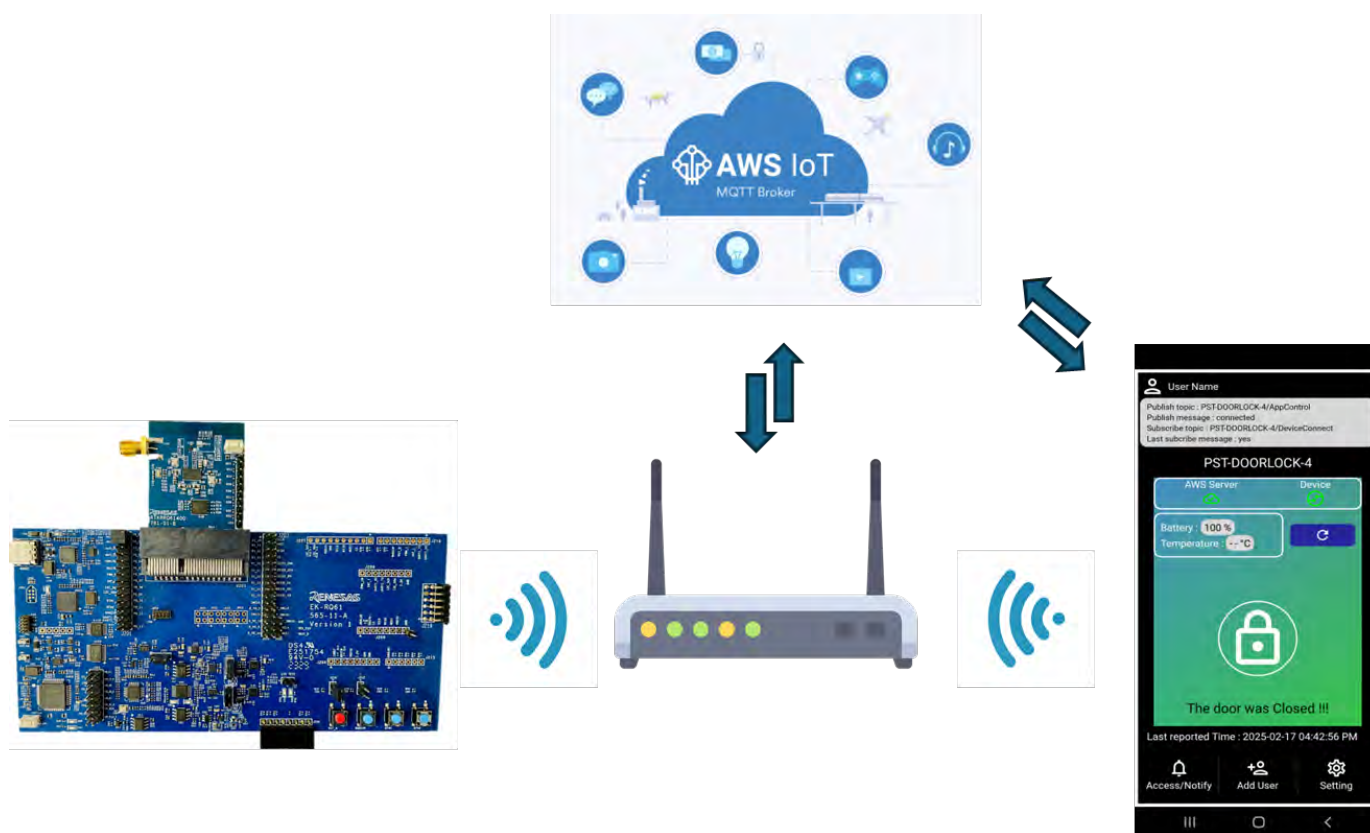
Figure 1. Architecture of AWS IoT reference application
