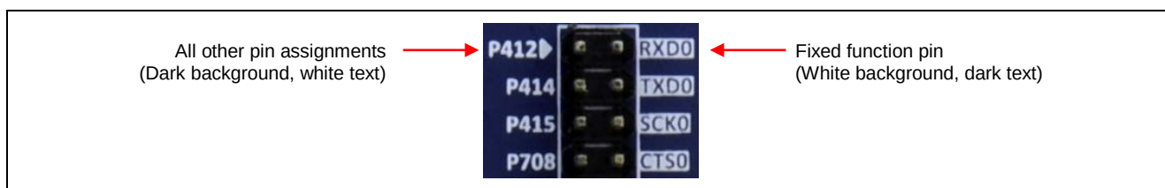
Figure 22. Fixed Function Pin Label Example
