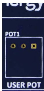
Figure 26. User Potentiometer on the Target Board (Top)
