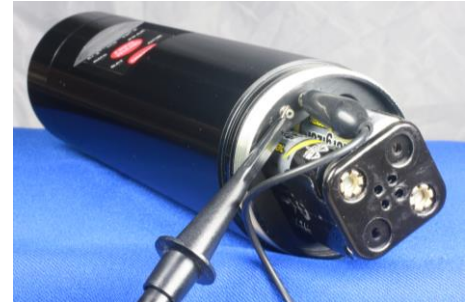
Figure 6: Probe connected to the test point pins
