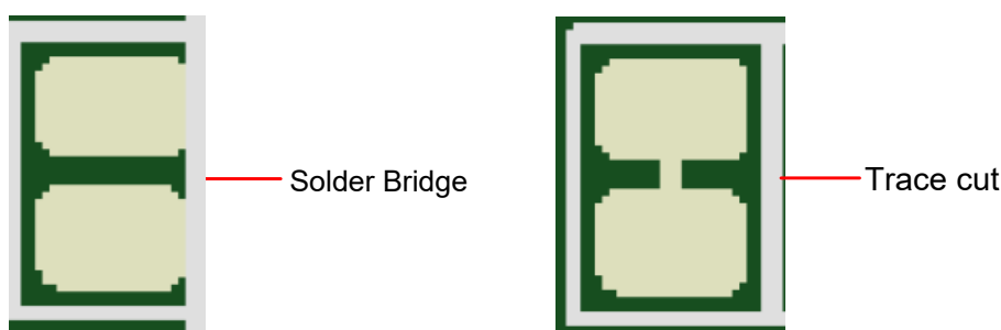
Figure 6-1 Solder Bridge and Trace Cut
