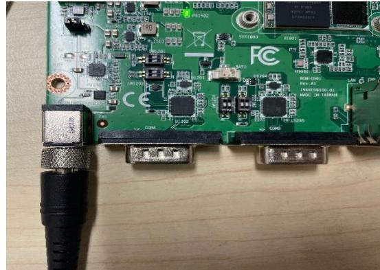
7 When switching on the power, the green LED indicator on BOT side of the board will light up to indicate that the board has booted up normally.
