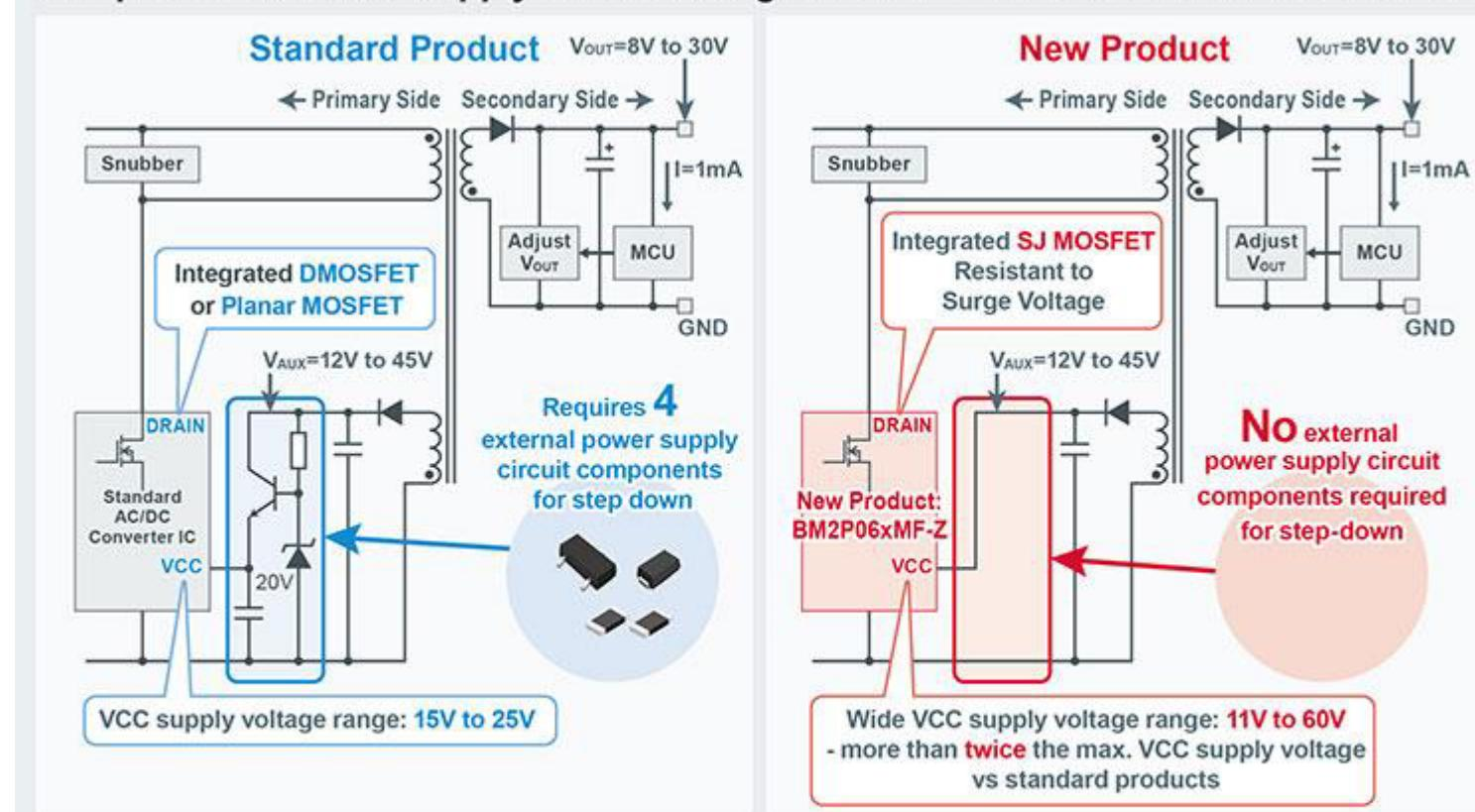
High VCC supply voltage combined with the SJ MOSFET featuring superior breakdown tolerance contributes to higher reliability
