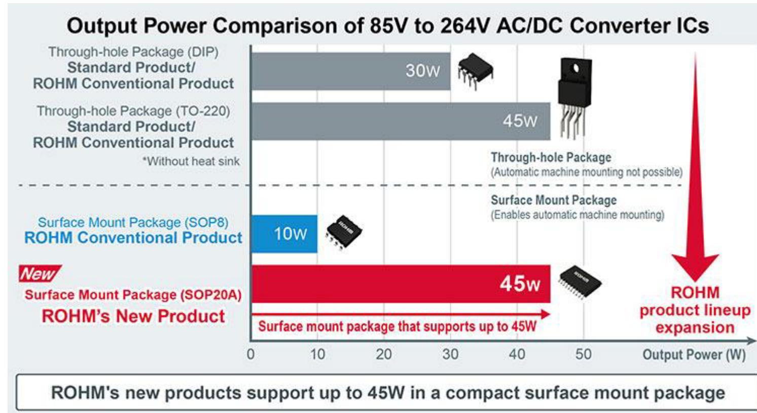
Compared to general products with equivalent performance, automatic mounting contributes to lower factory mounting costs. Moreover, ROHM is able to reduce standby power by over 90% along with the number of power supply circuit components by four, contributing to greater power savings and higher reliability in applications.
