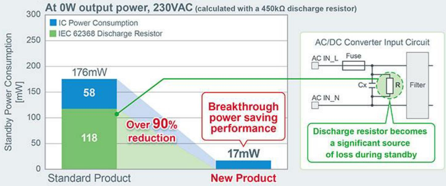
The BM2P06xMF-Z series eliminates the need for a discharge resistor while enabling further power savings through low standby power control technology
