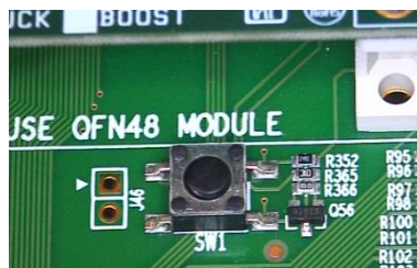
Figure 114: R365 (10 k \Omega ) Added Next to Reset Button
