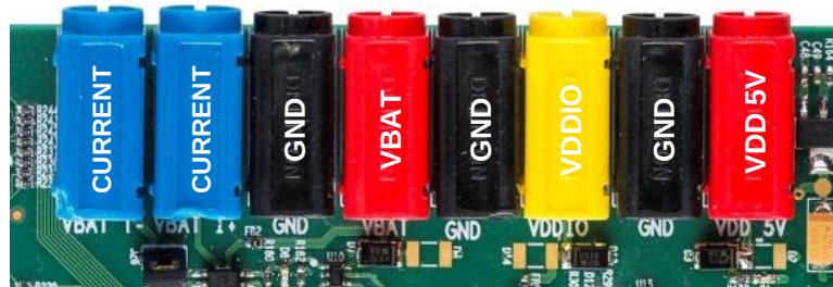
Figure 4: PLT Hardware Power Connections
