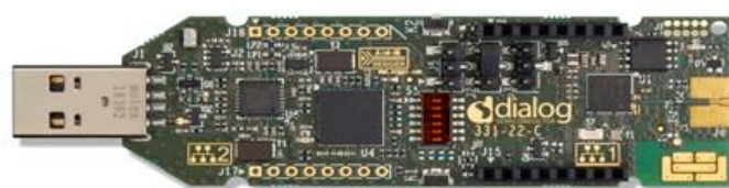
Figure 23: DA14695 USB Kit HW Components with External Antenna
