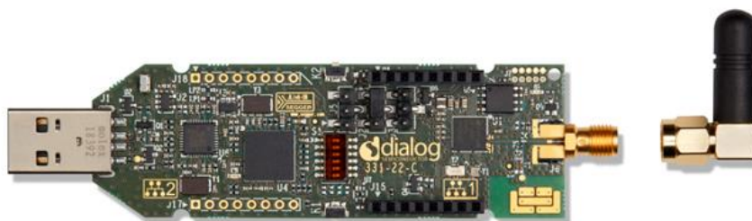
Figure 23: DA14695 USB Kit HW Components with External Antenna
