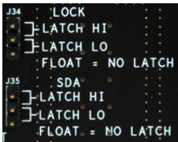
Figure 7. Lock Pin and SDA Pin Latch Control
