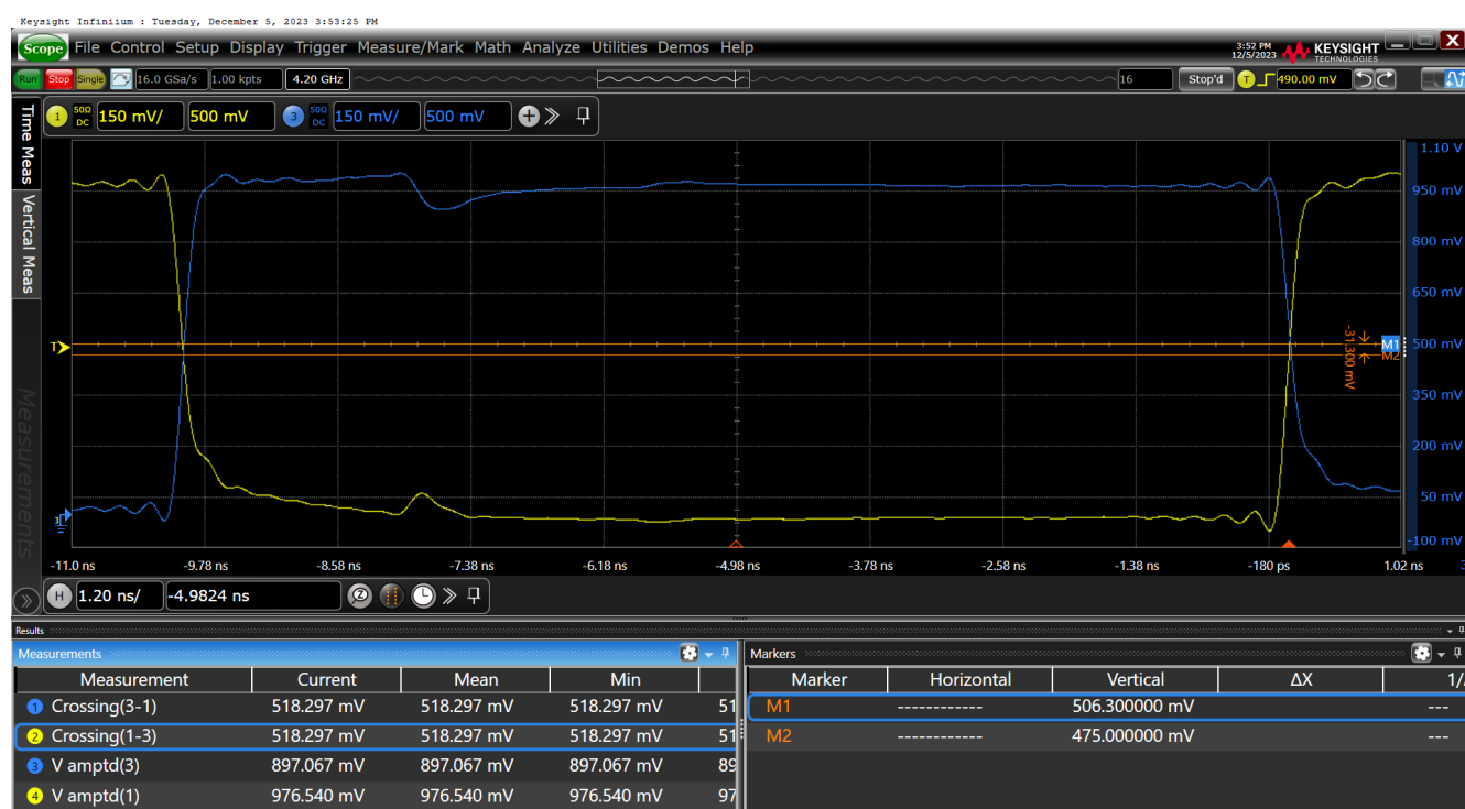
Figure 18. Vcross-HCSL Internal Termination SWING = 900mV on nOUT
