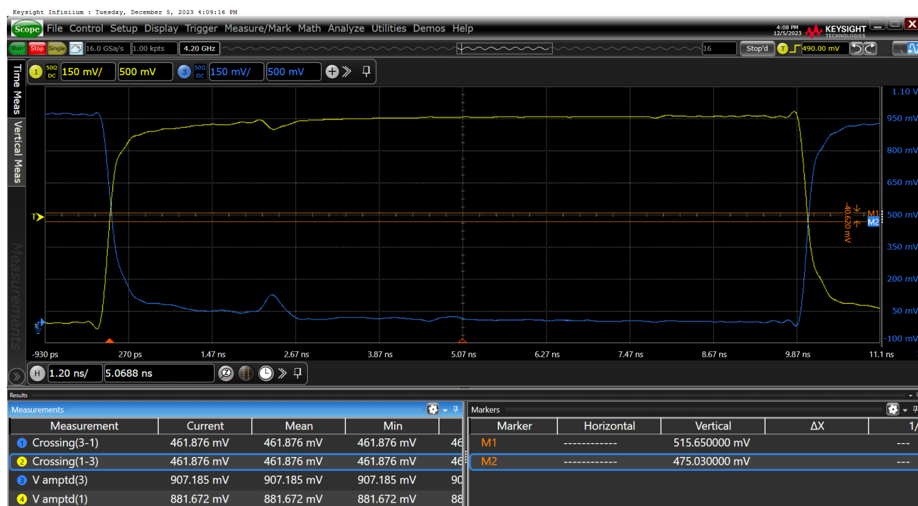
Figure 33. Vcross-HCSL External Termination SWING = 950mV on OUT11
