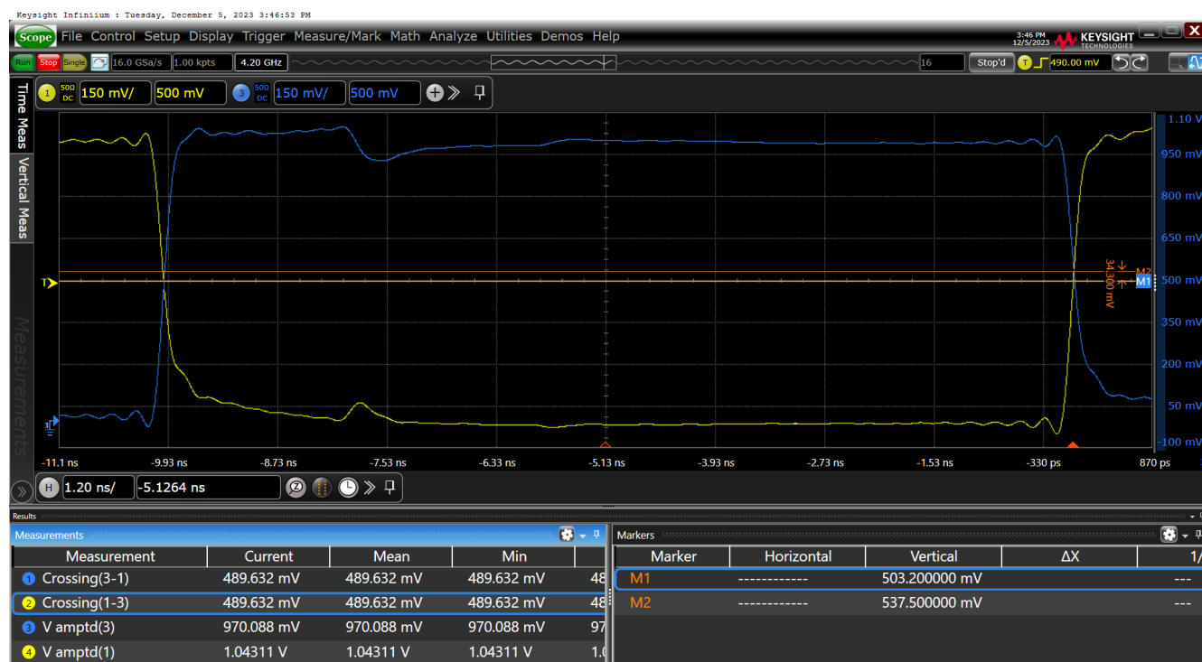
Figure 21. Vcross-HCSL Internal Termination SWING = 950mV on OUT11
