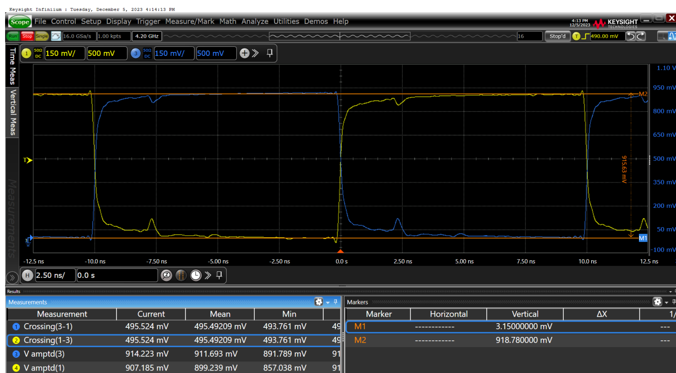
Figure 26. Vovs–HCSL External Termination SWING = 850mV on nOUT11
