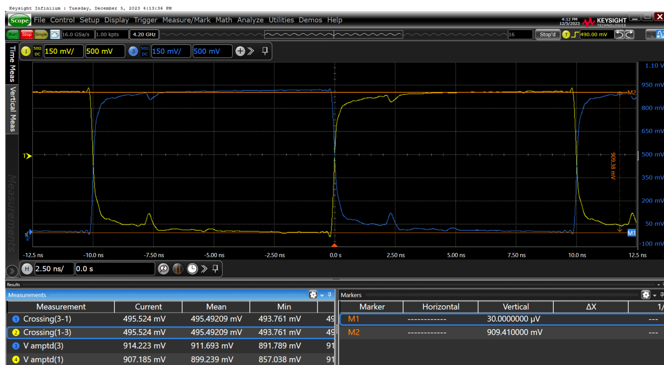
Figure 25. Vovs–HCSL External Termination SWING = 850mV on OUT11
