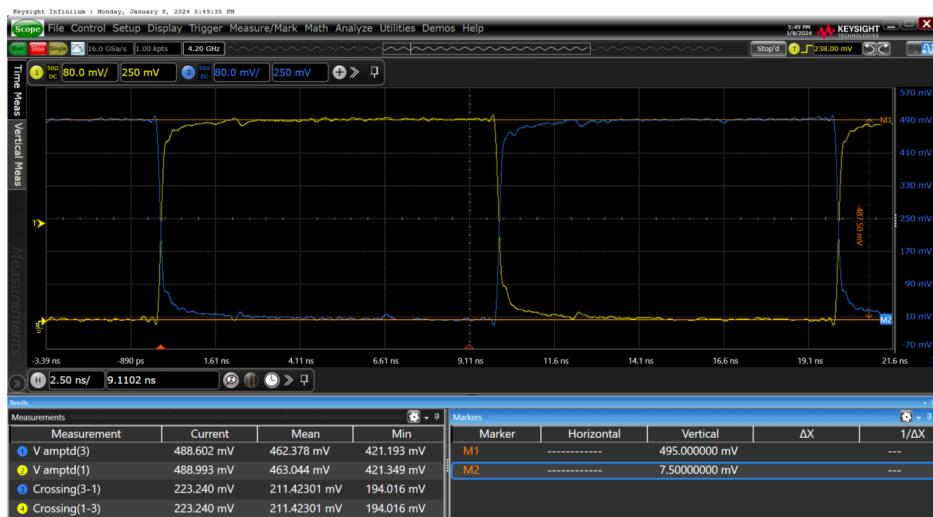
Figure 41. Vovs-HCSL Dual-Termination SWING = 900mV on nOUT11
