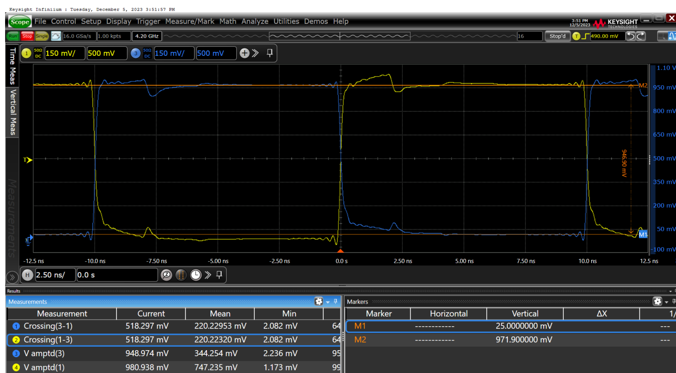
Figure 16. Vovs-HCSL Internal Termination SWING = 900mV on OUT11
