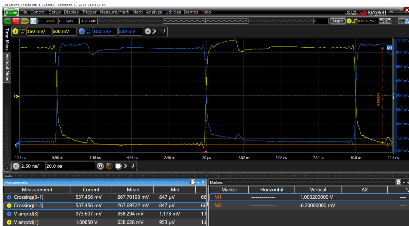
Figure 20. Vovs–HCSSL Internal Termination SWING = 950mV on nOUT11
