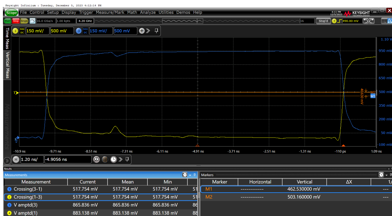
Figure 30. Vcross-HCSL External Termination SWING = 900mV on OUT11
