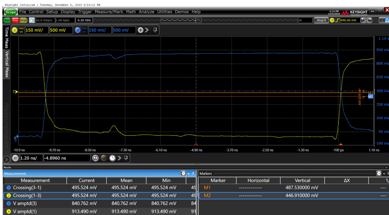
Figure 27. Vcross-HCSL External Termination SWING = 850mV on OUT11
