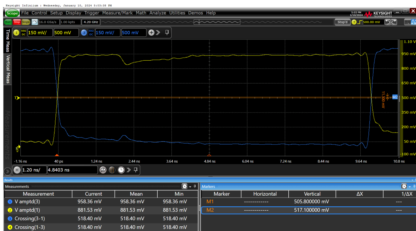
Figure 12. Vcross-HCSL Internal Termination SWING = 800mV on OUT11
