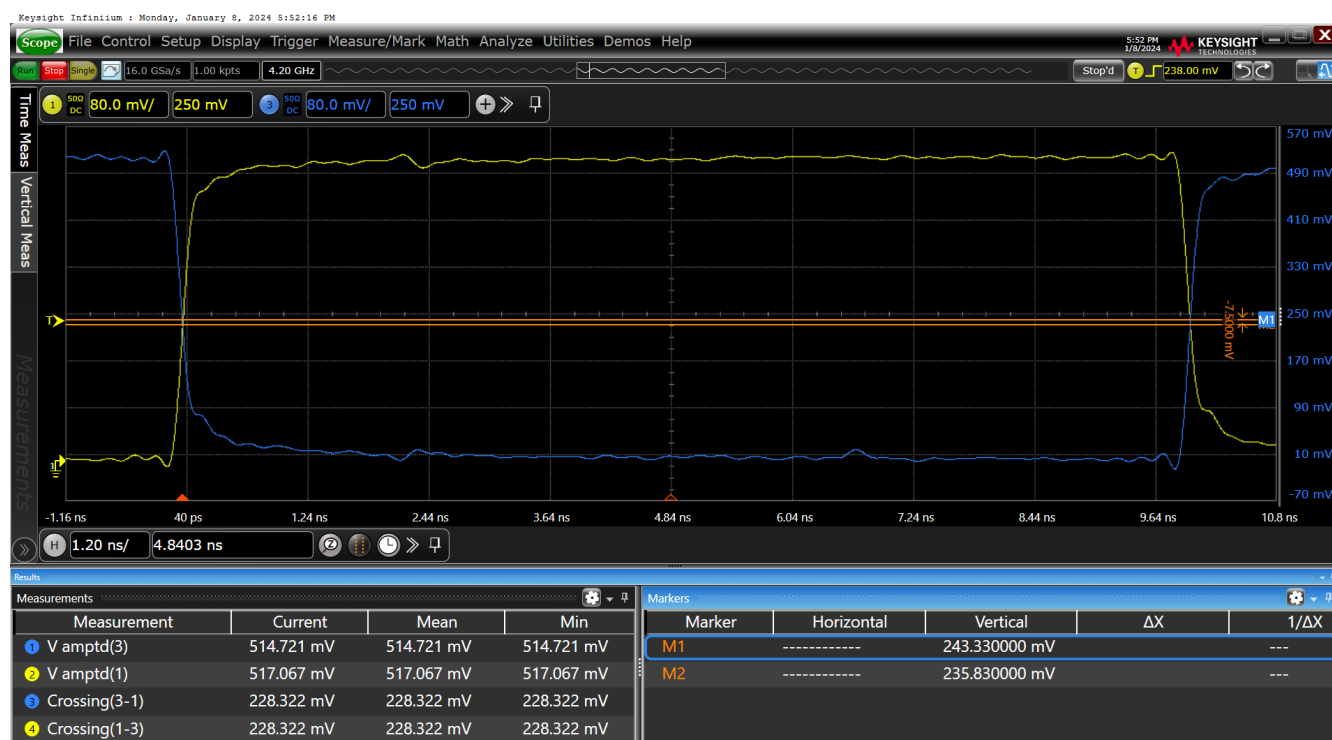
Figure 45. Vcross-HCSL External Termination SWING = 950mV on OUT11
