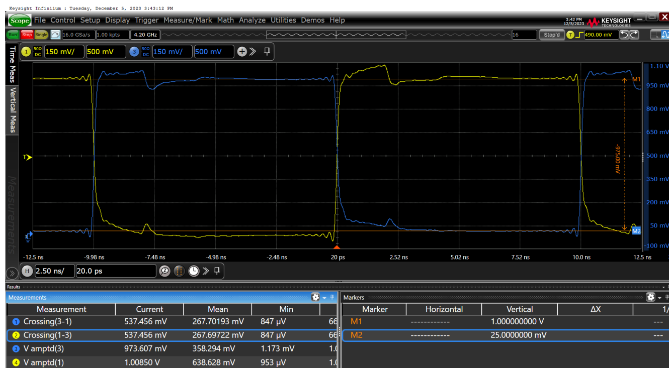
Figure 19. Vovs–HCSSL Internal Termination SWING = 950mV on OUT11
