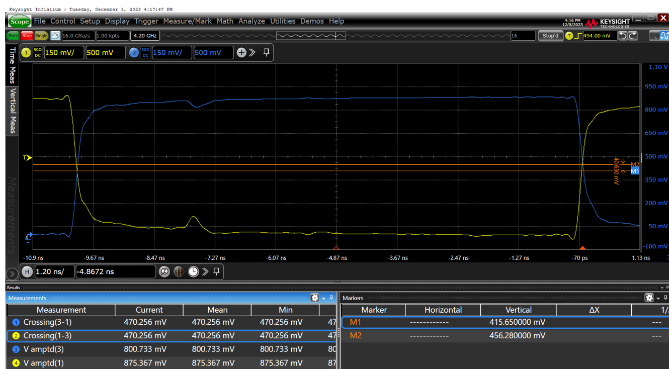
Figure 24. Vcross-HCSL External Termination SWING = 800mV on OUT11
