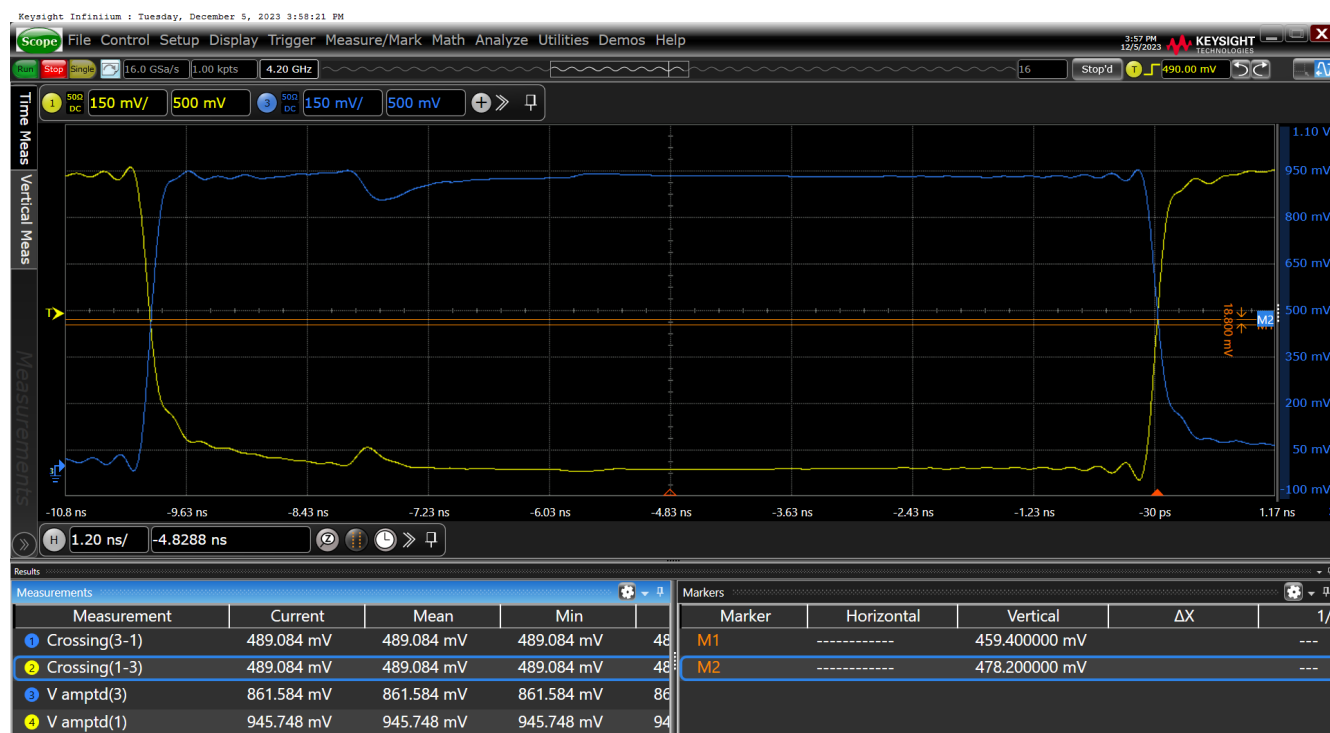
Figure 15. Vcross-HCSL Internal Termination SWING = 850mV on OUT11
