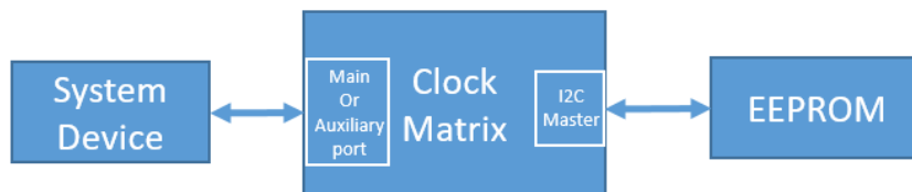
Figure 10. Programming the EEPROM through ClockMatrix
