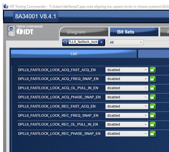
Figure 9. DPLL Channel 0 Fast Lock Settings for Master
