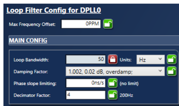
Figure 22. DPLL Channel 0 Loop Filter Configuration for Line Card
