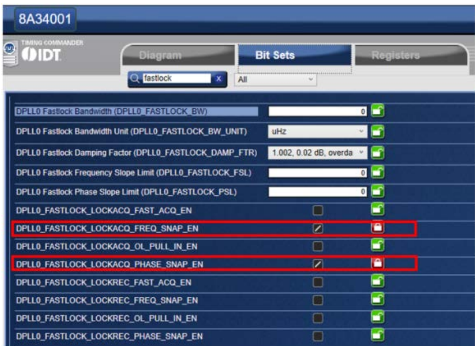
Figure 6. Enabling Frequency and Phase Snap for DPLL0 to Fast Lock to 1PPS Input
