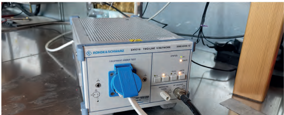
Fig. 10.12: LISN for AC and DC supply lines
