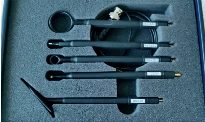
Fig. 10.3: Set of E-field and H-field sniffer probes
