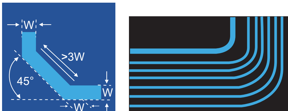
Fig. 4.17: Use 45^\circ or rounded track corners to reduce capacitive coupling interference
