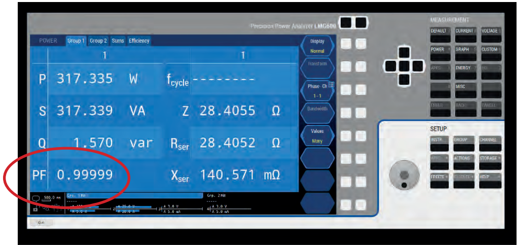
Fig 9.1: A power analyzer display showing a power factor (PF) figure of 0.99999
