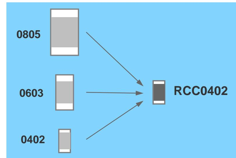
This is an example of a design change that can significantly reduce the component size from a standard 0805 to the RCC0402, rated to 125mW and 75V maximum operating voltage. This represents approximately 80% PC board space saving in addition to the superior thermal cycling performance with 3000 cycles capability for the RCC0402 versus 1000 cycles for the standard 0805.
