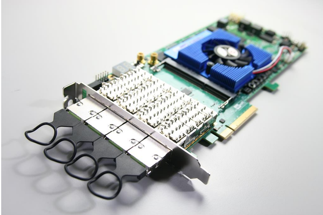
Figure 8-4 Four QSFP+ Loopback Fixtures Installed
