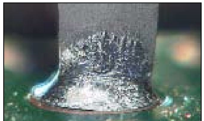
Figure 2. Lead Free Solder Lift-Off [5].
