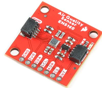
The ENS160 sensor operates from 1.71<sub>VDD</sub> to 1.98<sub>VDD</sub> voltage range, 1.71V to 3.6V<sub>VDDIO</sub> voltage range, and -40°C to 85°C temperature range. This sensor uses an I<sup>2</sup>C interface and is immune to humidity and ozone. The ENS160 sensor offers outputs such as eCO<sub>2</sub>, TVOC, and AQI compliant with worldwide Indoor Air Quality (IAQ) standards. Typical applications include building automation, smart home, and HVAC.
