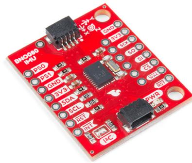
The SEN-14686 VR IMU breakout board is also equipped with two I<sup>2</sup>C Qwiic connectors to make interfacing with the tiny, QFN package a little easier. This board operates at a 1.65V to 3.6V voltage range and features 3Mbps UART, rotation vector, gaming rotation vector, geomagnetic rotation vector, and 1.5° gravity angle error.
