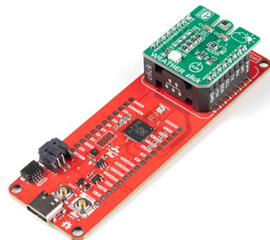
The RP2040 board is supports both C/C++ and MicroPython cross-platform development environments. This board features 264kB of embedded SRAM in six banks, six dedicated IO for SPI Flash, and thirty multifunction GPIO. The RP2040 mikroBus starter kit includes SparkFun RP2040 mikroBUS development board, MIKROE weather click, SparkFun micro OLED breakout (Qwiic), 100mm flexible Qwiic cable, and USB 3.1 cable A to C.
