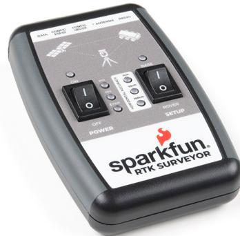
The RTK surveyor is a Bluetooth® enabled multi-band GNSS receiver based on the ESP32 from Espressif and the ZED-F9P from u-blox. The users can flip the switch to have 300mm approximate accuracy out of the box and 18mm accuracy with RTCM corrections. The RTK surveying kit comes in a handy carrying case to protect the most expensive bits. This kit works with common GIS software, including SW Maps, SurvPC, Field Genius, and any GIS software that supports NMEA over Bluetooth.
