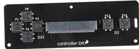
The controller:bit connects to the micro:bit via an edge connector in the center of the board. This creates a handy way to swap out micro:bits for programming, while still providing reliable connections to all of the different pins on the micro:bit. The back of the board includes poke home connectors that correspond to each button on the controller:bit, allowing to use external parts to control a game or robot.
