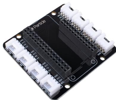
The grove shield for particle mesh requires minimal wiring and no soldering. The sensors, displays, and actuators can be plugged into the shield via the grove cable, and the project can be coded.
