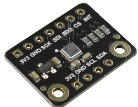
The ENS160 air quality sensor features a built-in algorithm, accurate output, automatic baseline correction, 3.3V power supply voltage, and 29mA working current. This module is used in air purification, environment pollution detection, electrical appliances, and building automation.
