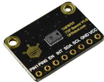
The TMF8701 sensor offers a high dynamic range and operates in either a proximity mode (1cm to 10cm) or a ranging mode (10cm to 60cm) for detection sensing. This sensor can make highly accurate distance measurements within  $\pm 5\%$  and can operate in the dark and in the presence of sunlight. The TMF8701 sensor outputs data through an I<sup>2</sup>C fast-mode communications interface and an integrated microcontroller.
