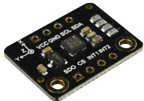
The triple-axis accelerometer features a 3.3V operating voltage, 8-bit data output, 10000g high shock survivability, and I<sup>2</sup>C/SPI interface. This accelerator also features two programmable independent interrupt engines that are able to recognize dedicated inertial events. The triple axis accelerometer can be used in high-speed impact detection and recording, free-fall detection, and automobile collision test.
