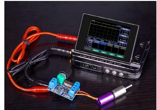
The MDP-XP includes a display control module and a digital power supply module. This system is controlled by an STM32 smart chip which allows for editing parameters and upgrading firmware at any time.
