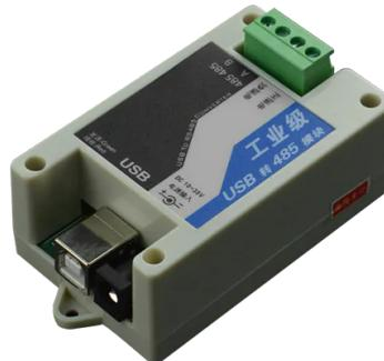
The USB to RS485 converter comes with built-in 15KV ESD protection and a maximum of 600W lightning surge protection. This converter adopts a self-recovery fuse + TVS protection circuit in terms of over-current and over-voltage protection to extend the service life of the module. The USB to RS485 converter features plug-and-play, hot-swappable, and built-in lightning surge protection.
