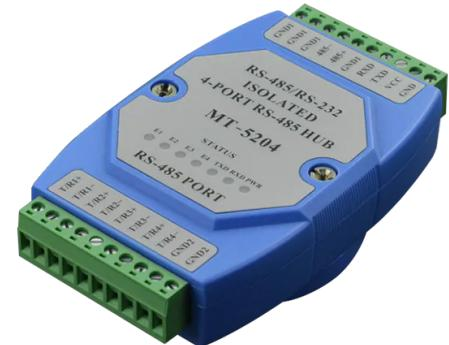
The RS485 opto-isolated hub has a transmission that reaches up to 115.2Kbps. This hub provides a star RS485 bus connection, and each port has short-circuit and open-circuit protection. The RS485 opto-isolated hub can provide more than 1200m transmission distance in RS485 working mode. This hub features  $9V_{DC}$  to  $30V_{DC}$ /150mA working voltage supply, 2500V isolation voltage, twisted pair or shielded wire transmission mode, and 10-position pluggable terminal blocks on both sides.
